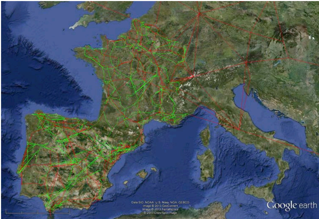
Figure 6 Initial network considered for the power systems of Portugal, Spain and France and the equivalent corridors among the rest of the EU countries
